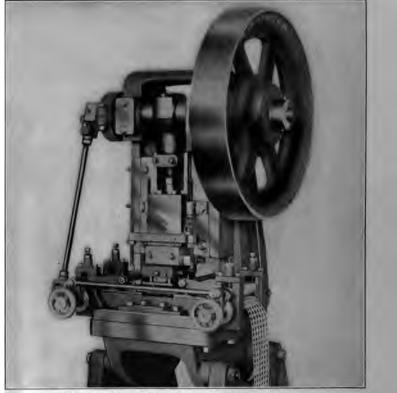
Fig. 3. Press Equipped with Double-roll Feed
